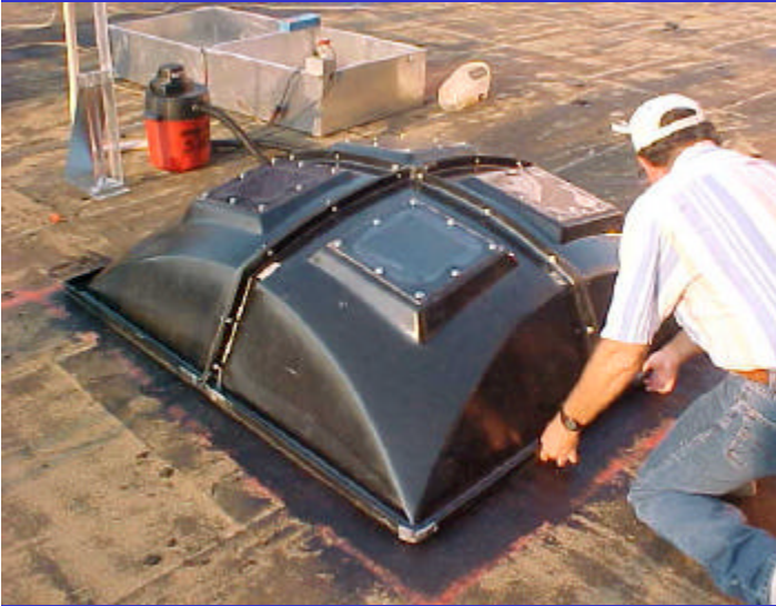
Uplift Test Apparatus
